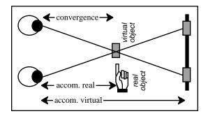
For see-through displays, it is possible to design dynamically compensating optics so that the accommodation depth always matches the convergence depth of the graphical object. However, if several different objects are presented, then the optics would have to track the convergence distance of the viewer's eyes in order to eliminate the effects of Accommodation - Vergence Conflict and Accommodation Mismatch.
