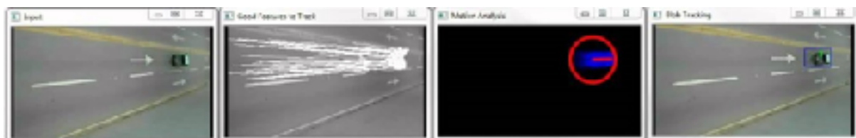
Figure 2: Example of a background subtraction algorithm for automatic traffic analysis. Image obtained from (Ferreira 2016).
