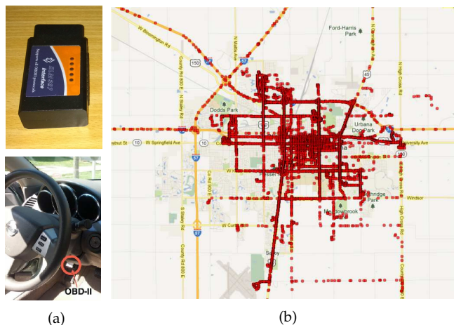
Fig. 2: (a) Deployed OBD-II to bluetooth adaptor; (b) Coverage map for the paths on which data were collected.
