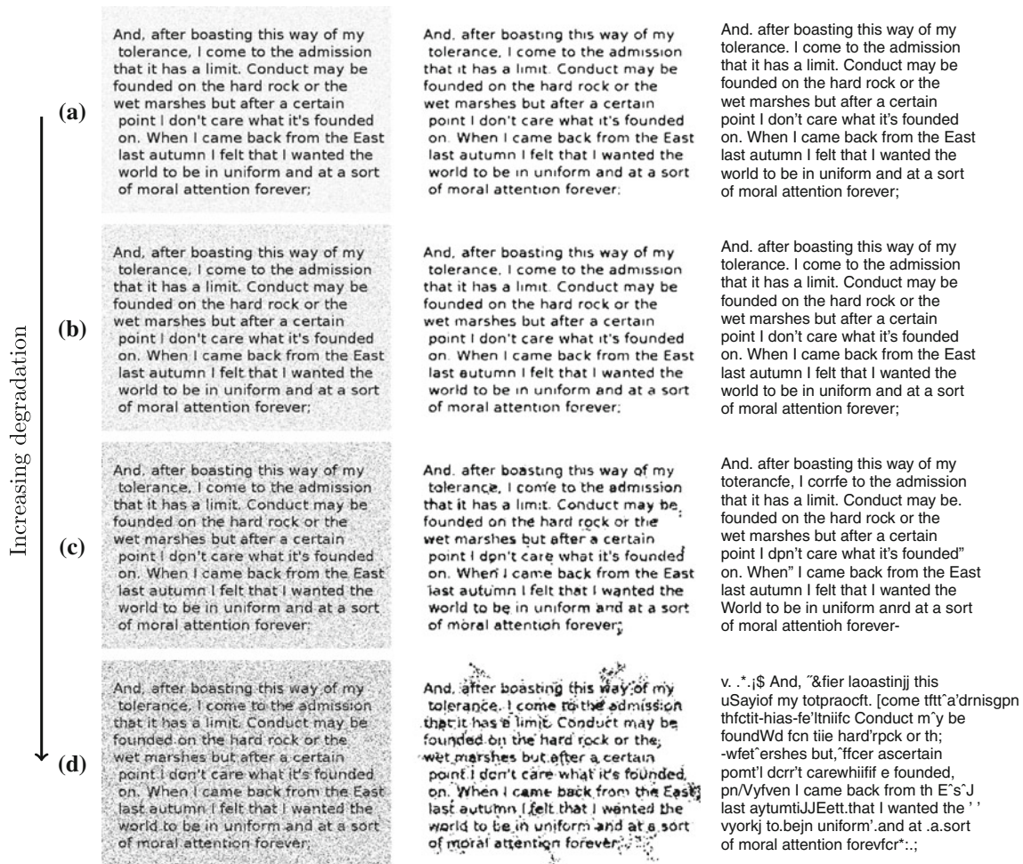
Fig. 14 Gaussian white noise. Left column Input image. Middle and right columns binarization and OCR results for various level of Gaussian white noise degradation: a \sigma_N = 10/255 , b \sigma_N = 20/255 , c \sigma_N = 30/255 , and d \sigma_N = 40/255 . See text in Sect. 3.2 and Table 1 for details
