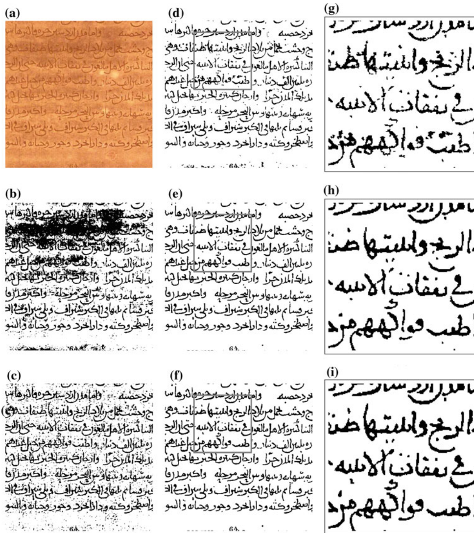
Fig. 19 Sample image from the Juma Al Majid Center for Cultural Heritage dataset (Dubai): a input image, b binarization obtained using Otsu’s method, and c binarization obtained using Sauvola’s method. The middle column shows two intermediate results of the proposed method:
