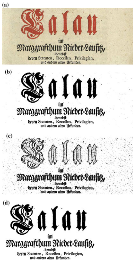
Fig. 23 Image P03 from the DIBCO'09 test dataset: a Input image, b binarization results obtained using Otsu's method, c binarization results obtained using Sauvola's method, and d binarization results obtained using the proposed method
