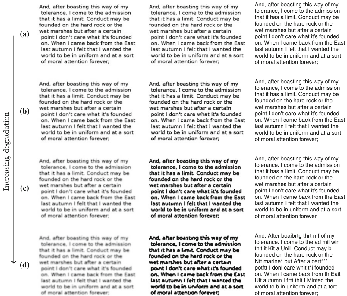
Fig. 13 Gaussian blurring. Left column Input image. Middle and right columns binarization and OCR results for various level of Gaussian blurring: a \sigma_B = 0.5 and k = 5 , b \sigma_B = 1.0 and k = 7 , c \sigma_B = 1.5 and k = 11 , and d \sigma_B = 2.0 and k = 13 . See text in Sect. 3.2 and Table 1 for details
