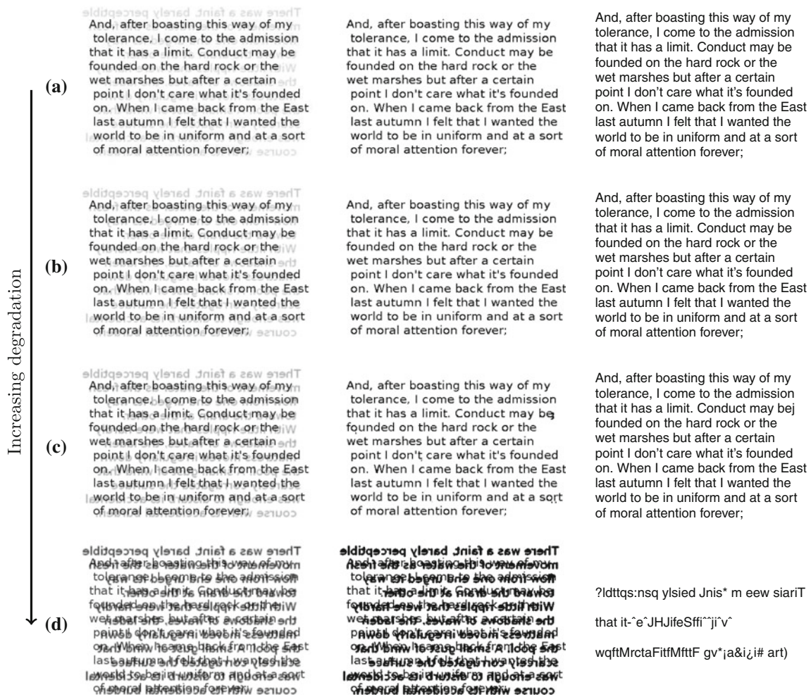
Fig. 12 Bleed-through degradation. Left column Input image. Middle and right columns Binarization and OCR results for various level of degradation: a d = 0.0390 , b d = 0.0552 , c d = 0.0782 , and d d = 0.2218 .
