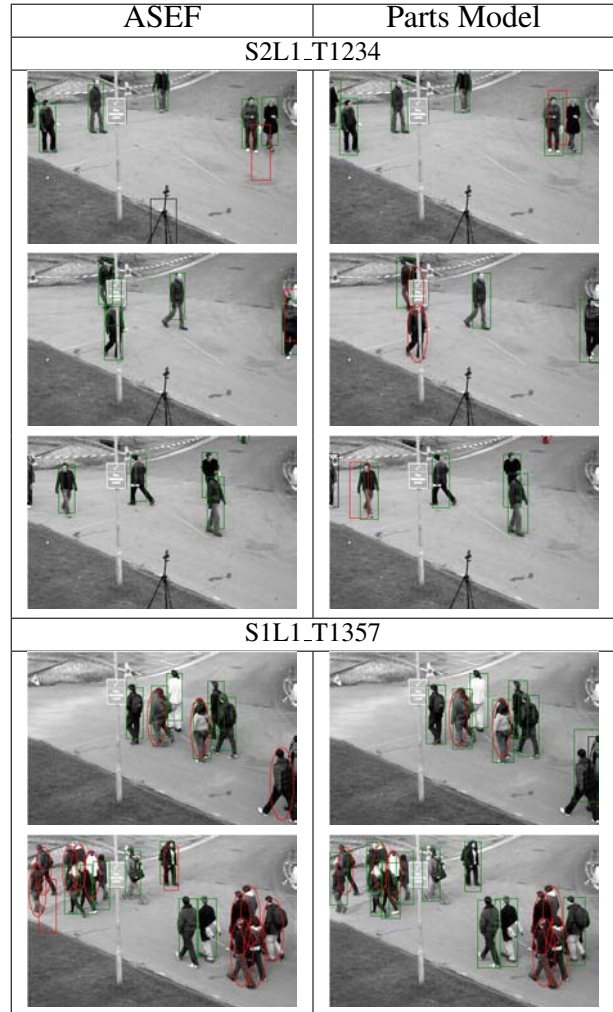
Figure 7: This figure shows some interesting detection challenges in the PETS dataset. Green rectangles indicate successes, red rectangles indicate false detections, and red ellipses indicate missed detections. From top to bottom: example false detections from people walking in close proximity, occlusion from the background, partial occlusion from by people, total occlusion by people, and densely packed groups of people.
