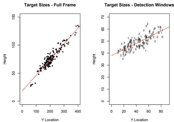
Figure 2: The left plot confirms that the height of people in the full frame can be approximated nicely using a linear model. This is expected given the approximately plainer ground. The right plot shows the height of those people in the rescaled detection regions. In the rescaled regions there is much less variation in the person height.
