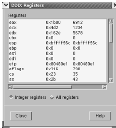
Figure C.6 Register Window after the single-stepping shown in Figure C.5.
