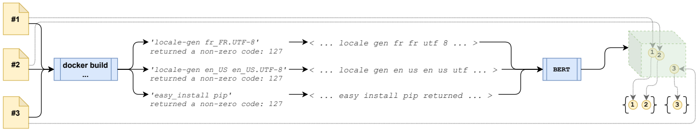
Fig. 4: Clustering Example. Starting with several broken Dockerfiles, SHIPWRIGHT clusters by extracting standard error logs, applying aggressive token splitting (we split on snake and camel case, as well as several operators that may occur in code snippets) and string normalization (we lowercase the input, clear large blocks of repetitive characters, like extraneous white space, and we strip certain special characters/unicode), and passing the resulting sequences to BERT. BERT takes the input sequences and produces vectors (shown as points in a high-dimensional space). SHIPWRIGHT uses that mapping, from failing build logs to points in a vector space, along with a clustering algorithm (HDBSCAN), to produce its clusters, shown in the bottom right of the figure. The final clustering process has the advantage of being semantics aware : BERT understands some of the nuances of the English language, and our clustering benefits from this capability.
