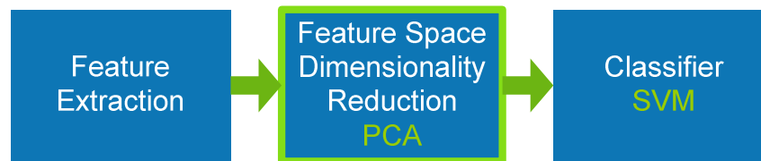
Figure 23. Face Detection Block Diagram - PCA Feature Space Reduction
