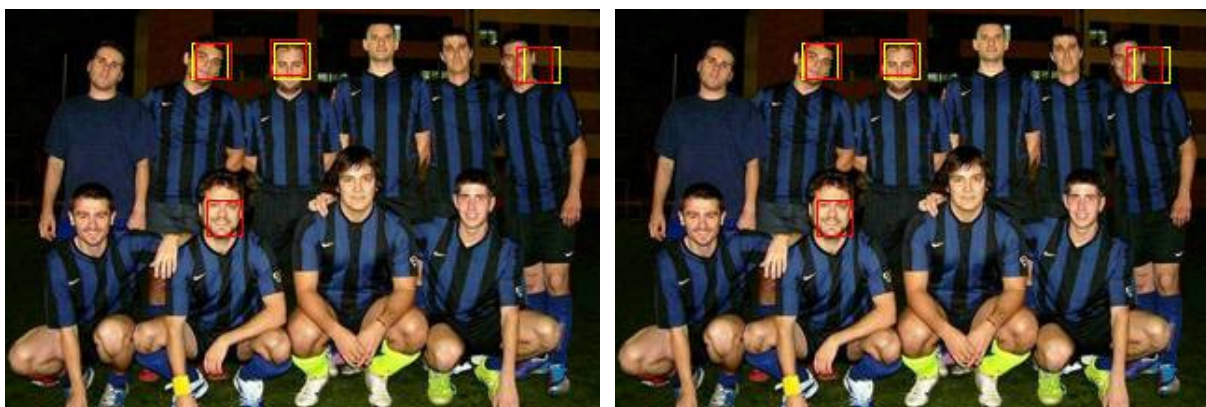
Figure 70. PCA Only Faces - ref image classification using BioID training set (19x19)
