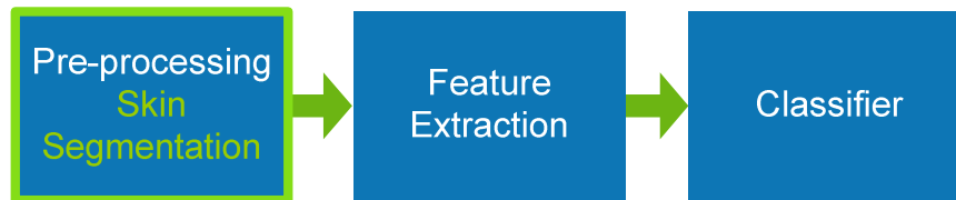
Figure 26. Face Detection Block Diagram with Skin Segmentation Pre-processing
