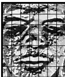
Figure 38. LBP_{(8,2)}^{u2} image example of size 126x147: 7x7 blocks of 18x21 pixels
