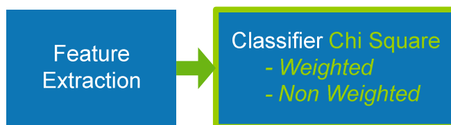
Figure 14. Face Detection Block Diagram - Chi Square Classifier
