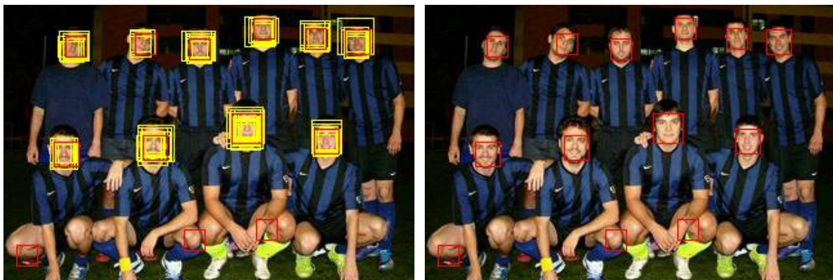
Figure 69. PCA Only Faces - ref image classification using GTAV Internet training set (16x16)
