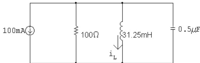
$$i_L(0) = 20 \text{ mA}, \quad i_L(\infty) = -100 \text{ mA}$$
