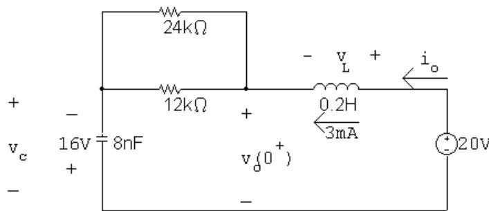
$$12 \text{ k}\Omega \parallel 24 \text{ k}\Omega = 8 \text{ k}\Omega$$
