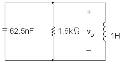
$$i_R(0) = \frac{60}{1600} = 37.5 \text{ mA}; \quad i_L(0) = 45 \text{ mA}$$
