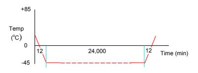
Cooling rate: $5 \,^{\circ}$ C/minTest temperature: $-45 \,^{\circ}$ C  $\pm 2^{\circ}$ CDwell time400hHeating rate: $5 \,$  oC/min to room temperatureSettle time:24hPass Criteria:Gain, bandwidth and centre frequency to remain unchanged after test
