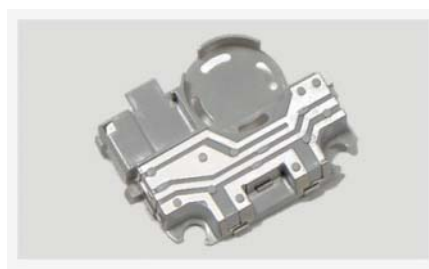
Figure 88: Ceramic Planar inverted-f-antenna (PIFA) and PIFA for a cellular phone
