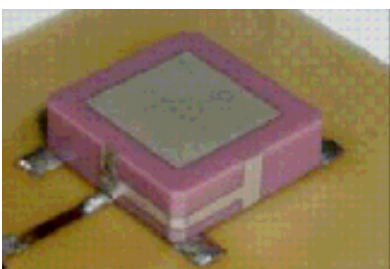
Figure 88: Ceramic Planar inverted-f-antenna (PIFA) and PIFA for a cellular phone
