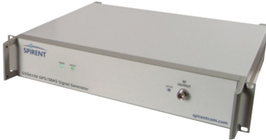
Figure 29: 1-channel GPS simulator
