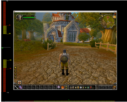
Figure 1 - Bars on the side and bottom of the screen give feedback to users about their tracking position. The green mark represents the player's position. For the vertical bar, if the green mark reaches the yellow area the character walks, and reaching the red area makes the character run. The top yellow and red areas represent moving forward, while the bottom area represents moving backward. The horizontal bar on the bottom of the screen represents the amount of rotation applied to the character, based on the distance from the center (position control).
