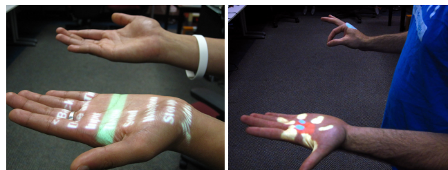
Figure 7. Left: Hierarchical menu navigation on the hand. Right: demonstration tattoo painting application.
