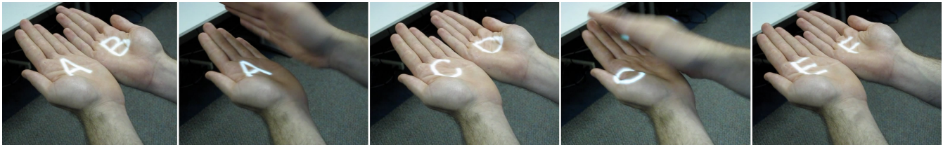
Figure 3. Two hands can create a book interaction metaphor. “Pages” can be turned by flipping the appropriate hand, which transitions the interface. Time advances from left to right.
