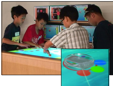
figure 2. Four children playing the KORC game on a custom-built three-sided multi-touch tabletop system. Visually tagged circular tokens are placed on the tabletop to identify players.
