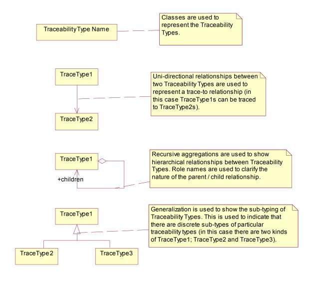
To fully understand the diagrams it is useful to know the implementation mapping used when implementing the definitions in RequisitePro. The table below explains how the diagramming notation can be mapped onto RequisitePro projects.
