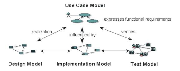
The figure shows the models and the implicit relationships between these models. The relationship between the models provides a level of traceability that is implicit to the development process.
