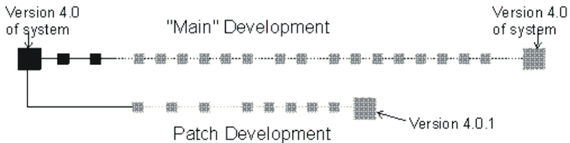
The development of a patch release is done in parallel with the main development project. Gray squares indicate future releases and baselines.
