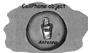
Object with one non-primitive instance variable— a reference to an Antenna object, but no actual Antenna object. This is what you get if you declare the variable but don't initialize it with an actual Antenna object.
