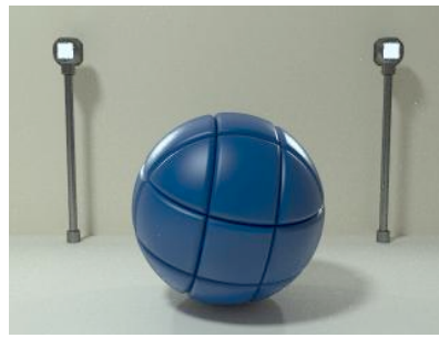
Krylon latex enamel #7205, True Blue. The enamel paint has been coated with a gloss-reducing finish Plasti-kote #33, Glass Frosting Spray.
