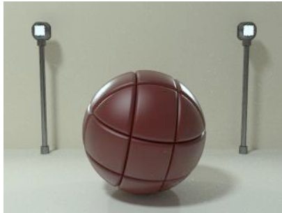
Dupli-color #T-345, Garnet Red. The lacquer has been coated with a gloss-reducing finish Plasti-kote #33, Glass Frosting Spray
