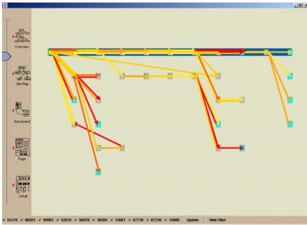
Figure 1: The WebQuilt visualization. Nodes represent visited web pages, and arrows represent the traffic between the pages. Entry pages are colored green, and exit pages cyan. Thicker arrows representing heavier traffic. Arrow color is used to indicate time spent on a page before transitioning, where the closer the arrow to red, the longer spent in transition. The designer's path is highlighted in blue. The slider interface along the left hand side allows the designer to zoom into the graph, viewing actual images of the pages users saw, and where they clicked.
