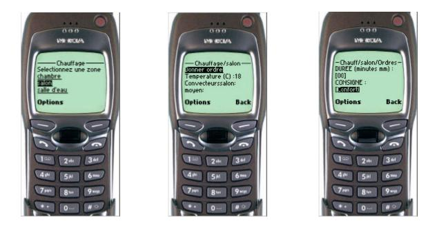
Figure 2. Modifying the temperature using a WAP-enabled mobile phone.
