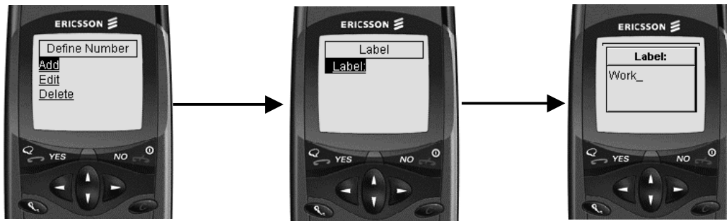
Figure 9.3. Pictures showing the extra step (middle card) when making a hyperlink ( Add ) to an input-field.
