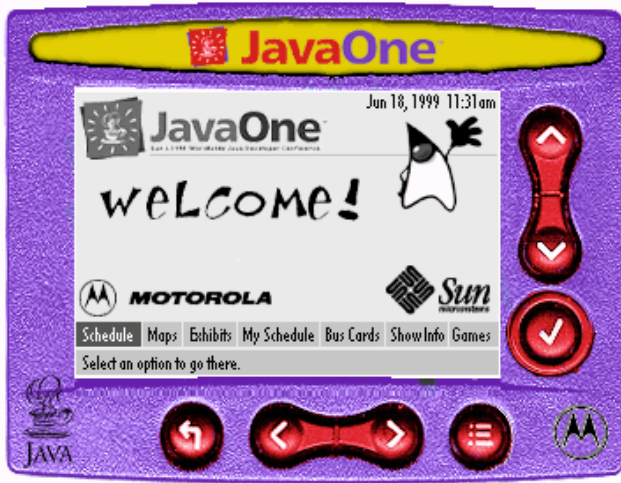
Illustration 2: An early version of the Home screen using a button bar to access the applications. This is shown on a mockup of the Garnet device which was not the final device used.
