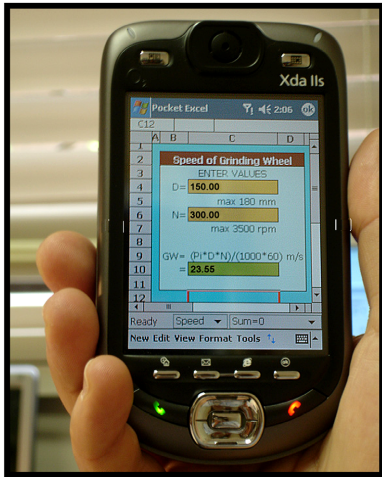
Fig. 3. “Speed of grinding wheel” analytical tool created by Jack with MS Excel.
