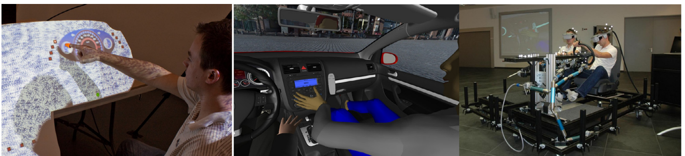
Fig. 3. Example of spatial augmentation of a car panel on the left (Porter et al., 2010). On the right a Virtual Reality system that tracks the user viewpoint to correctly render the content on the HMD (Salzmann & Froehlich, 2008).
