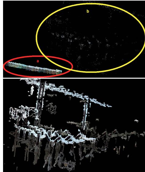
Figure 8. Top image shows the result of test case 304 after the initial reconstruction stage using Bundler. On the bottom, the results after the final dense reconstruction stage using CMVS. Observe cameras trajectory as almost a linear footage at the camera path (a).
