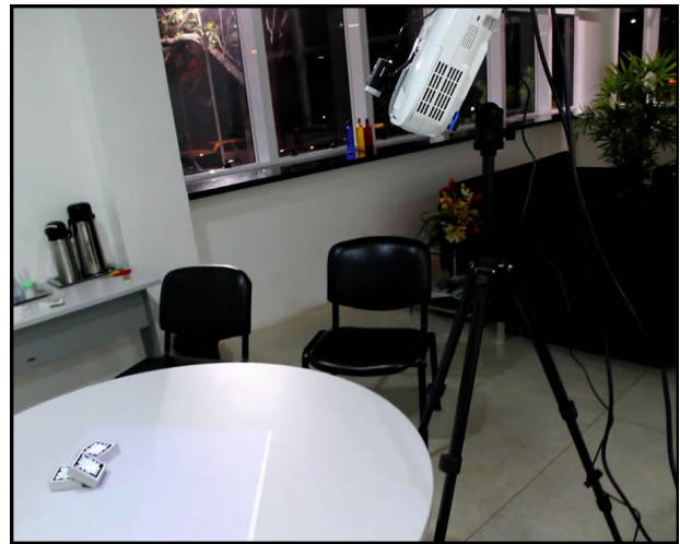
Figure 11. Camera-projector system setup, using a tripod. The projector illuminates the table where the children can use the system.
