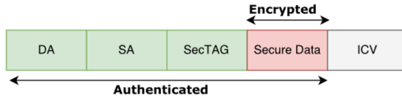
Figure 5.4: The MACsec Frame Format.
