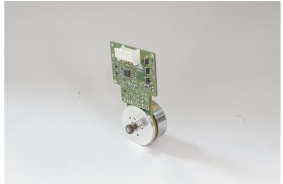
(b) Motor Maxon EC-45 Flat 50W
