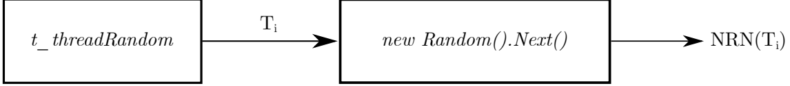
Figure 8: Only NRN(T_i) can be observed by the attacker - T_i is never revealed.
