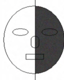
Figure 10. Division of a face into two sub images to handle the severe cases of half illuminated face
